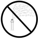
Make sure there are no sprinkler heads near the heat pump that will spray on or into the unit. **Sprinkler damage is not covered under the warranty agreement.** Make sure that sprinklers are placed at a sufficient distance away, so that normal wind will not carry the mist to the heat pump.
